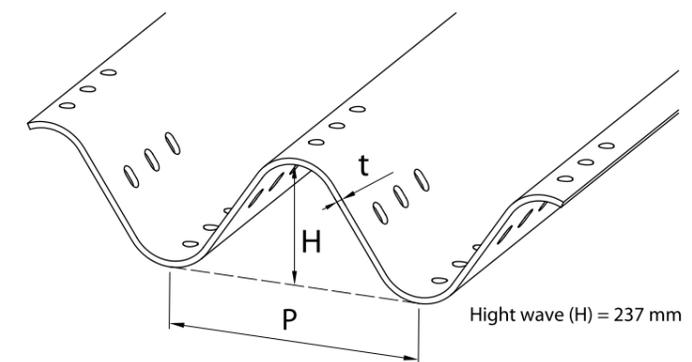
Fig. 1. Wave profile of UC plate
