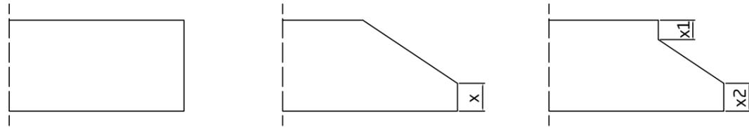
Fig. 6. End finishes of UltraCor®
