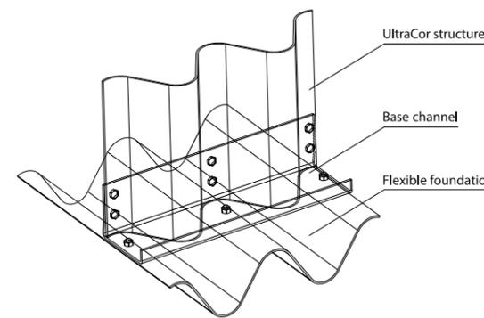
Fig. 8. Connection of UltraCor® structure with flexible footing
