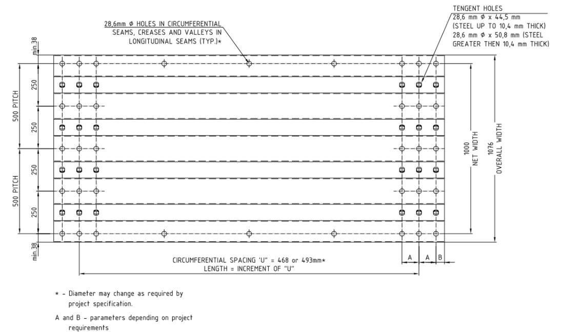
Fig. 3. Geometry of UltraCor plate.
