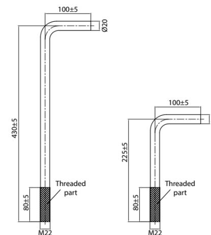
Fig. 4. Anchor bolts used to mount structure in foundation.
