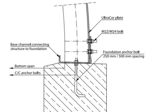
Fig. 9. Connection of UltraCor® structure with concrete footing
