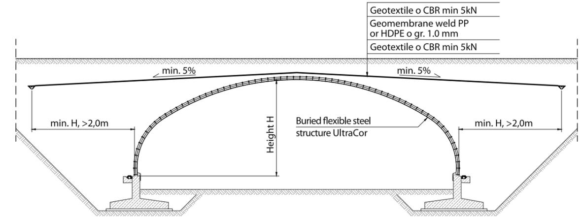
Fig 10. Scheme of rainwater protection
