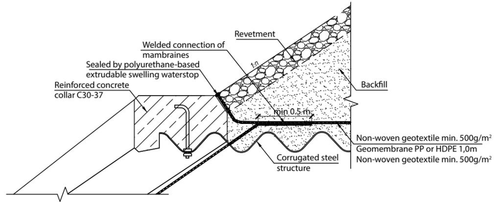
Fig 11. Detail of concrete collar with drip
