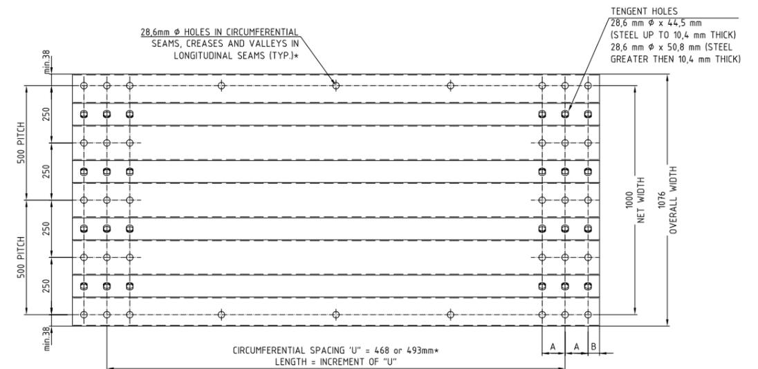
Fig. 3. Geometry of UltraCor plate.
