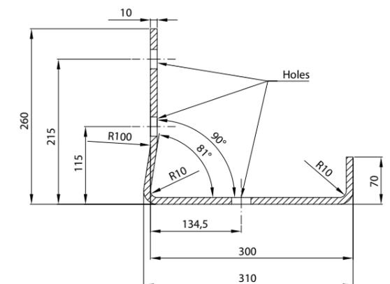
Fig. 5. Base channel used to connect structure to foundation.
